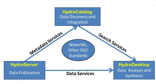
An online distributed system to support the sharing of hydrologic data from multiple repositories and databases via standard water data service protocols; software for data publication, discovery, access and integration. CUAHSI HIS: NSF support through 2012 (GEO)
